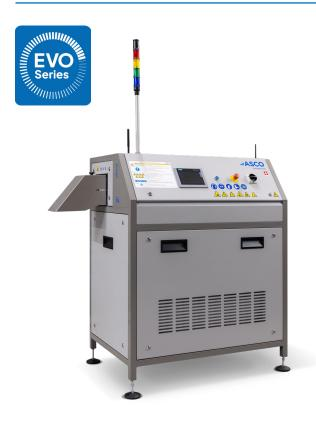
The **ASCO** Dry Ice Pelletizer P15 is a compact and powerful dry Ice machine. Having an adjustable production capacity of 100 - 150 kg/h (220 - 331 lb/h) it meets the demands for higher dry ice quantities plus quality and flexibility in the daily working process.
